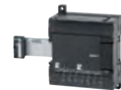
■ Analog I/O Unit CP1W-MAD11 • Analog inputs: 2 (resolution: 6,000) • Analog outputs: 1 (resolution: 6,000)
